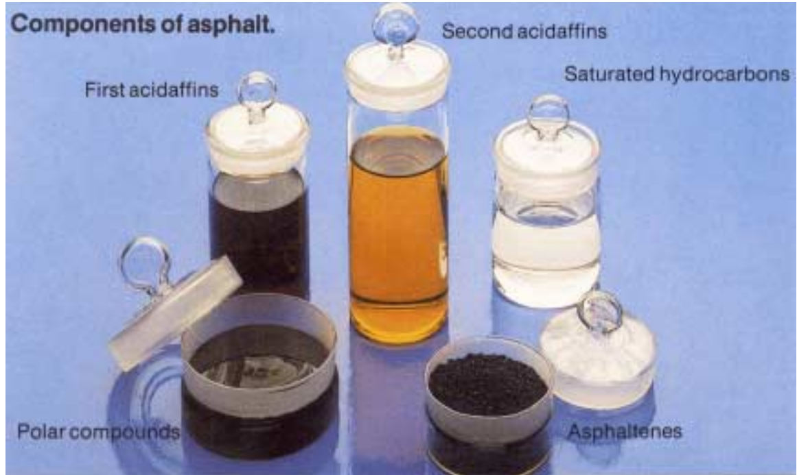
Figure 1. Asphalt Binder Fractions, Asphaltenes and Maltenes.
